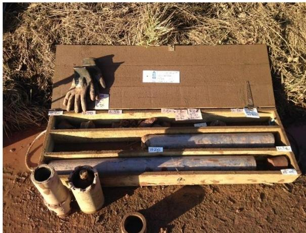
Bore hole samples for testing
